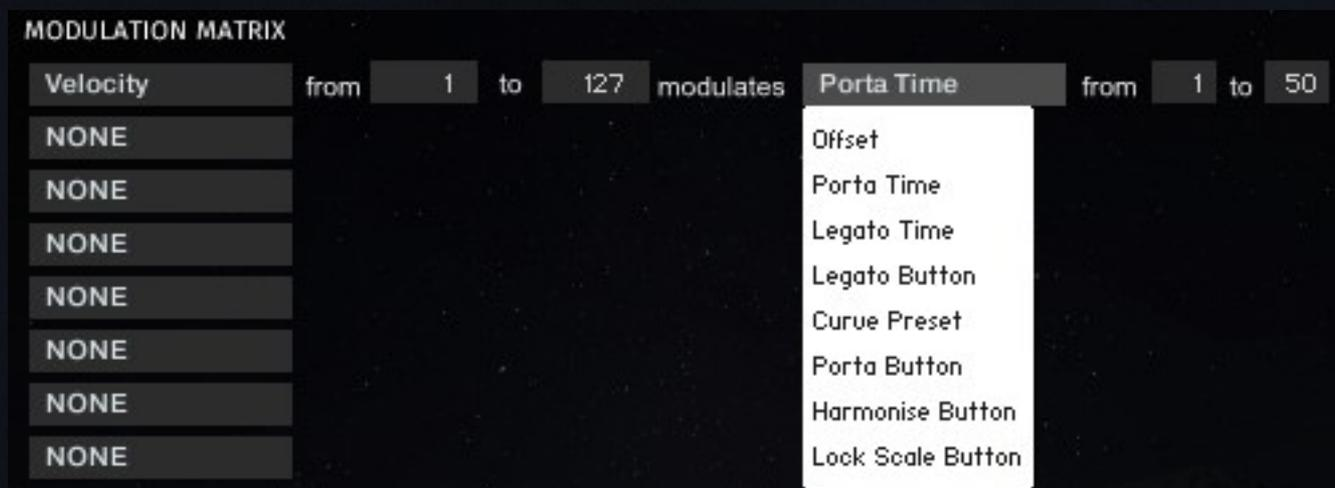
This list will show different items depending on the source. The line is now set up, the only things left to choose are the exact values. The source menu and the destination menu are constant, however the other controls will work in 1 of 4 ways: Standard, button, keyswitch or special.
